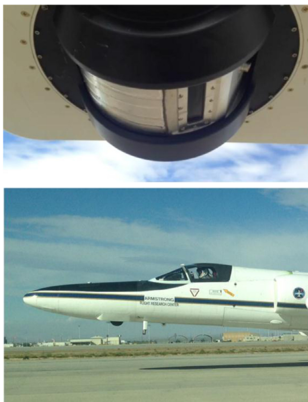
Fig. 10. Upper panel: the rotating drum containing the AirMSPI-2 camera is shown mounted to the nose of the ER-2 aircraft. The optical viewport (rectangular slit) through which the camera observes is shown. Lower panel: AirMSPI-2 is shown mounted on the underside of the aircraft in the nose cone just ahead of the extended pitot tubes.
