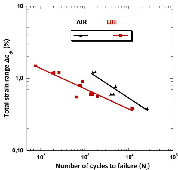
**Fig. 4.** Evolution of the total strain range with the number of cycles to failure of T91 steel fatigued in air and LBE at 350°C
