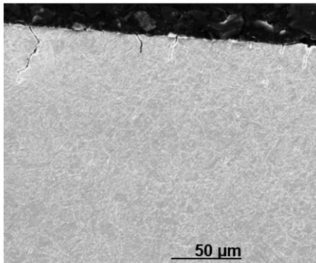
**Fig. 6.** Observation of short cracks in T91 steel fatigued in air at 350°C and  $\Delta \epsilon_t = 1.2\%$
