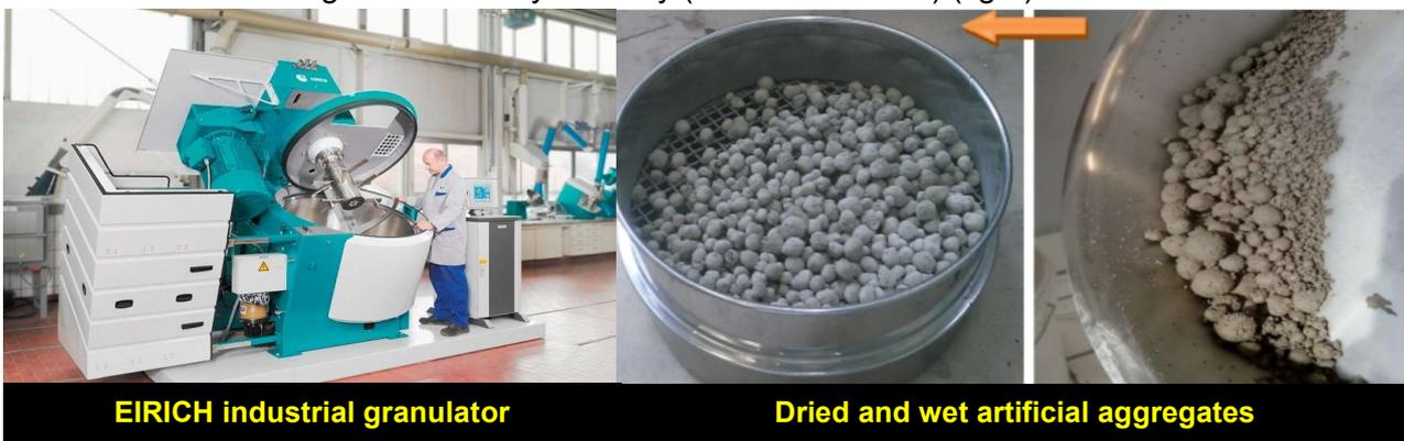
**Fig.3 EIRICH granulator and sediment-derived aggregates**
