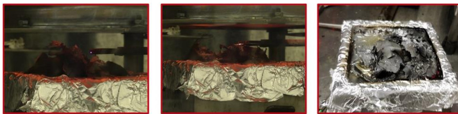
Fig. 8. Pictures taken of PI when subjected to 50 \text{ kW/m}^2 at 1541 s (left), before removing sample (middle), and after the removal of the sample from the heat source (right).
