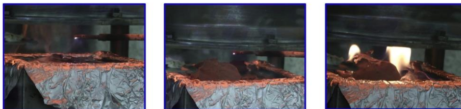
Fig. 9. Pictures taken of PI when subjected to 60 \text{ kW/m}^2 at different times during the experiment: 60 s (left), 360 s (middle), 401 s (right).
