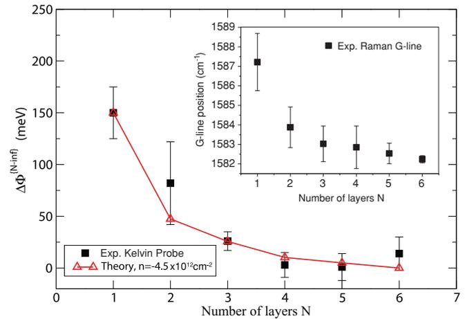
FIG. 4. (Color online) Work function differences as a function of the layer thickness (full squares), extracted by histogram analysis of the acquired Kelvin probe data. (Inset) Raman G-line shift. Triangles indicate *ab initio* DFT calculations of the work functions for a doping level of  $n = -4.5 \times 10^{12} \text{ cm}^{-2}$ .
