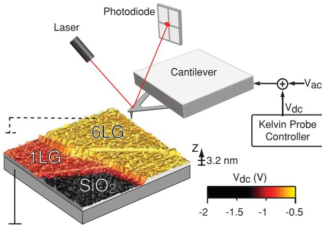
FIG. 1. (Color online) Schematic illustration of the Kelvin probe force microscopy setup used to investigate graphene flakes resting on  $\text{SiO}_2$ . In the three-dimensional rendering of the topography brighter areas indicate higher recorded contact potential difference ( $V_{dc}$ ) (see scale bar). A lower  $V_{dc}$  i.e. higher work function is recorded over areas of single-layer (1LG) than six-layer (6LG) regions.
