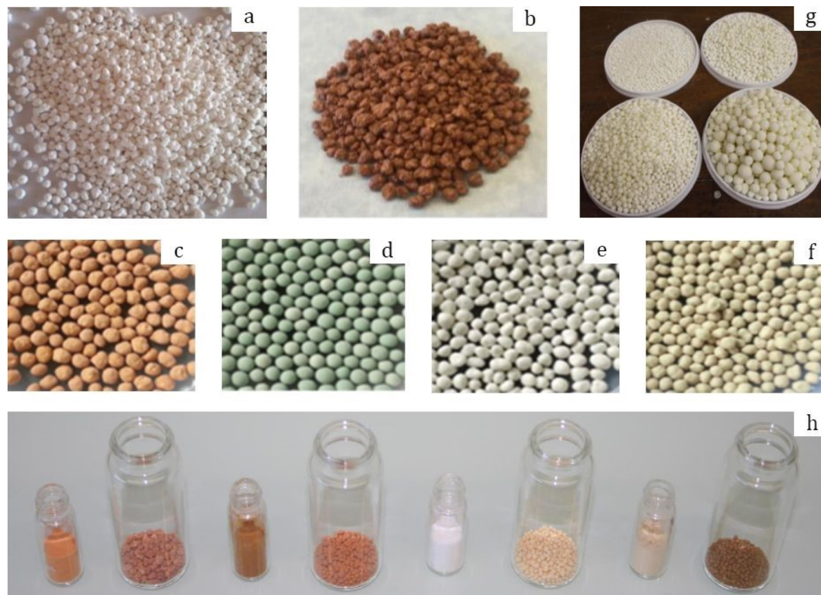
Fig. 5 Photographs of: MIL-160 granules (a) prepared by Permyakova et al. [67]. Copyright 2017 Wiley. MIL-100 granules (b) prepared by Martins et al. [69]. Copyright 2020 American Chemical Society. MIL-100 (c), MIL-101 (d), UiO-66 (e), and UiO-66-NH 2 (f) containing 5 wt.% MRA binder prepared by Valekar et al. [57]. Copyright 2017 The Royal Society of Chemistry. UiO-66 granules (g) prepared by Ren et al. [73]. Copyright 2017 Elsevier. MIL-100, MIL-127, UiO-66, UiO-66-NH 2 granules (h, from left to right in big vessels) with their corresponding powders in small vessels prepared by Chanut et al. [71]. Copyright 2016 Wiley.
