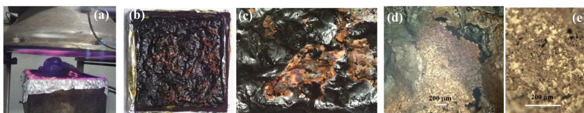
50 Figure 16. (a) Char formation as seen in MLC experiment in C2-TPU. (b) Sample collected at 51 the onset of experiment (c) red patches on the char on the char collected at 'onset' (d,e) 52 Focussed images on red patches. 53 54 55 56 57 58 59 60
