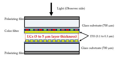
Figure 2. Schematic localization of LCs in the LCD panels.
