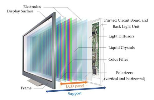
Figure 1. Structure of an LCD-TV module (from [13]).
