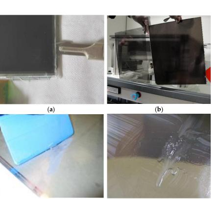
**Figure 3.** The opening stages of an LCD panel giving access to LCs. (**a**,**b**) Manual opening of the sandwiched glass plates using a scalpel. (**c**) Separation of the two glass plates, on the left-hand side, front of the panel consisting of color filters and black matrix; on the right-hand side, back side. (**d**) Collected LCs molecules with translucent and slightly viscous aspects.
