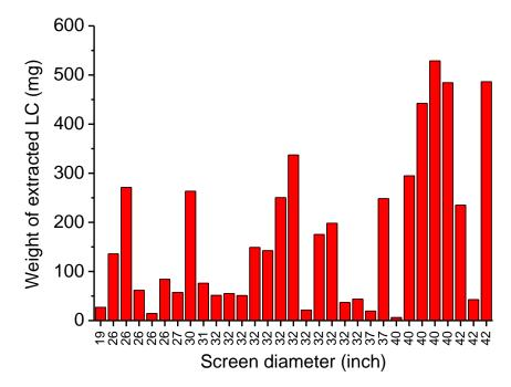
Figure 4. Weight of LCs mixtures extracted manually from 31 EOL-LCD panels.
