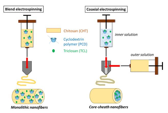
**Figure 1.** Schematic presentation of the preparation of monolithic and core-sheath nanofibers based on chitosan, cyclodextrin polymer, and triclosan.
