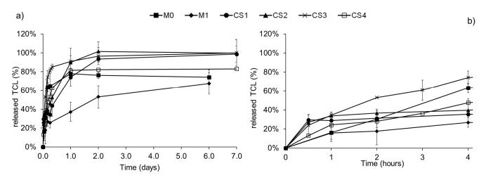
**Figure 5.** Triclosan release profiles in PBS at pH 7.4 at 37 °C from monolithic and core-sheath nanofibers (a) in a time period of 7 days and (b) within the first 4 h.
