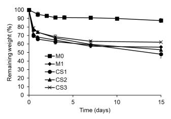
**Figure 4.** Weight loss at pH 7.4 at 37  $^{\circ}$ C within 15 days of degradation of monolithic and coresheath nanofibers.
