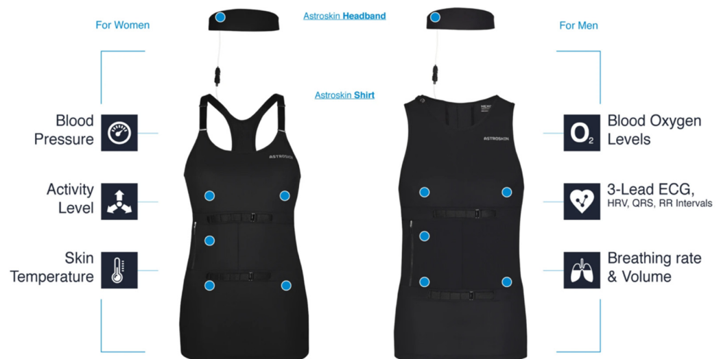
Figure 6. Healthcare e-textile system prototype design (“Astroskin” shirt by Carre Technologies Inc. (Hexoskin)) [43] (Reprinted with permission from Ref. [43]. Copyright 2021 Carre Technologies Inc.).
