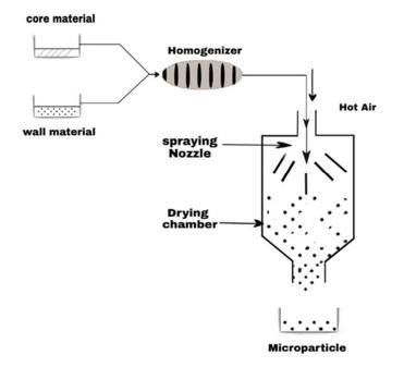
Figure 6. Schematic representation of the spray-drying microencapsulation process.
