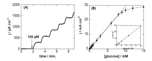
**Figure 4.** (**A**) Amperometric response curve of CQDs/Cu<sub>2</sub>O-modified GCE polarized at +0.55 V vs. Ag/AgCl upon successive additions of glucose (100  $\mu$ M) in 0.1 M NaOH (up to a total of 500  $\mu$ M); (**B**) Calibration curve for CQDs/Cu<sub>2</sub>O-modified GCE electrodes for the determination of glucose. The inset corresponds to a calibration curve for glucose concentrations of 0–10  $\mu$ M.
