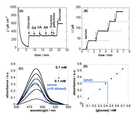
**Figure 5.** (**A**) Interference test of CQDs/Cu<sub>2</sub>O-modified GCE electrode in 0.1 M NaOH at +0.55 V with 100  $\mu$ M glucose in the presence 500  $\mu$ M dopamine (DA), uric acid (UA), ascorbic acid (AA), fructose, galactose; (**B**) current response to the addition of serum; (**C**) UV/Vis spectra of different concentrations of glucose as well as of the serum samples (ten times diluted) together with calibration curve (**D**).
