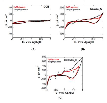
**Figure 3.** Cyclic voltammograms of (**A**) glassy carbon electrode (GCE); (**B**) GCE/Cu<sub>2</sub>O; and (**C**) GCE modified with CQDs/Cu<sub>2</sub>O by drop casting in 0.1 M NaOH aqueous solution in the absence (red) and presence of glucose (black, 100  $\mu$ M).
