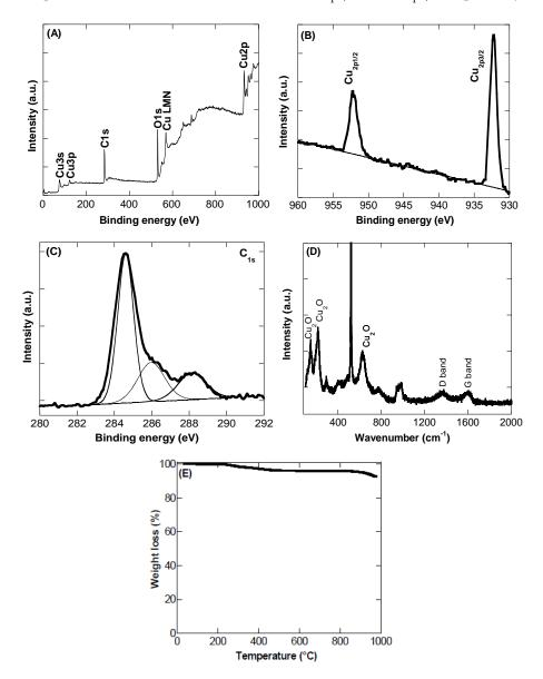
**Figure 2.** (**A**) X-ray photoelectron spectroscopy (XPS) survey spectrum; (**B**) Cu<sub>2p</sub> core level spectrum; (**C**) C<sub>1s</sub> core level spectrum; (**D**) Raman spectrum; (**E**) thermogravimetric analysis (TGA) thermogram of CQDs/Cu<sub>2</sub>O nanocomposite.
