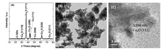
**Figure 1.** Characterization of carbon quantum dots loaded with copper oxide nanoparticles (CQDs/Cu<sub>2</sub>O NPs): (**A**) X-ray powder diffraction (XRD) pattern; (**B**) transmission electron microscopy (TEM) image; (**C**) high-resolution TEM (HRTEM) image.
