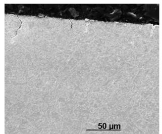
Fig. 6. Observation of short cracks in T91 steel fatigued in air at 350° C and  $\Delta \epsilon_r = 1.2\%$
