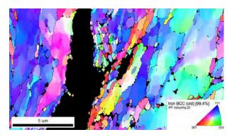
Fig. 10: IPF acquired near the crack tip in T91 fatigued in air at  $350^{\circ}$  C and  $\Delta\epsilon_{t}=1.2\%$
