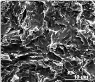
Fig. 9. SEM observation of the fracture surface between two striations of T91 steel fatigued in LBE at 350° C and  $\Delta \varepsilon_t$ = 1.2% showing brittle fracture
