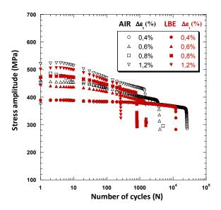
Fig. 3. Evolution of the stress amplitude with the number of cycles of T91 steel fatigued in air and LBE at 350°C
