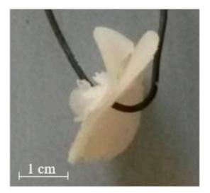
Figure 3. Picture of an AMY-based disk after 5h exposure to phosphate buffer pH 6.8.
